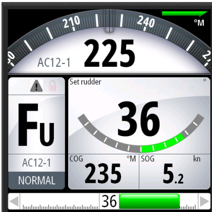
Follow-up mode with rudder setting, course and other nav data clearly displayed.
