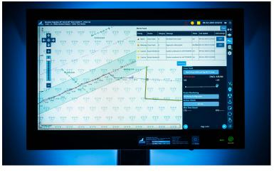
The 24-inch colour display, touch screen and PC is contained within a single panel PC. This operating system is ideal for compact installations.
