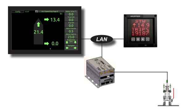
The new SKIPPER DL 21 is a speed log, working on the Doppler principle, providing Speed through water (STW) and Speed over ground (SOG) in 2 axis.
