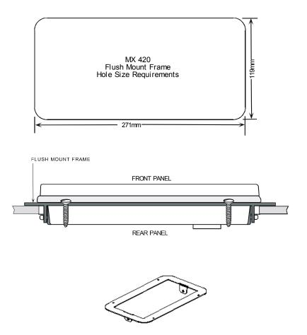
Figure 3.5 Optional Flush Mount Frame Installation
