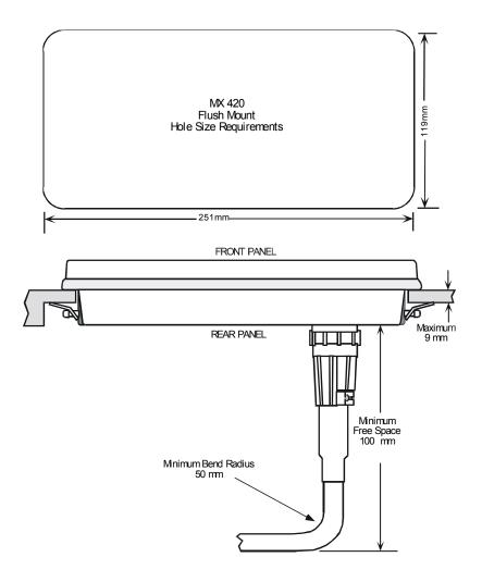
Figure 3.4 Standard Flush Mount and Cable Clearance
