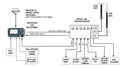
Figure 4.19 MX420/AIS/MKD CDU & MX531 (ATLAS) Transponder Block Diagram
