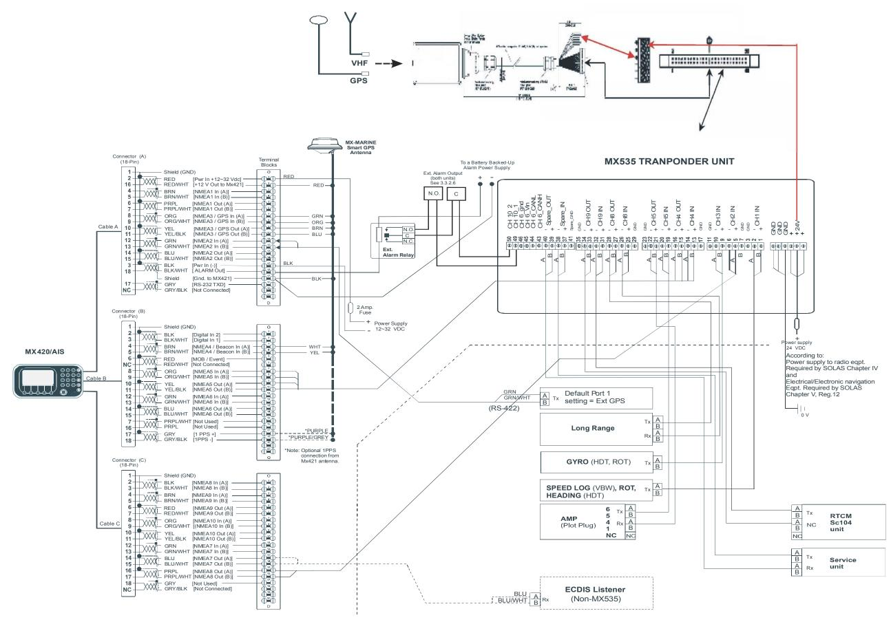
Figure 4.22 - MX420/AIS/MKD CDU & MX535 (NAUTICAST) Transponder System Wiring Diagram
