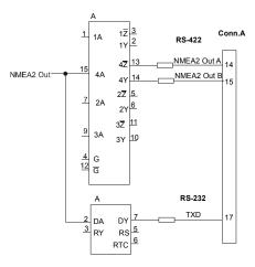
Figure 5.1 Port 2: RS- 422 / RS- 232 Port Schematic
