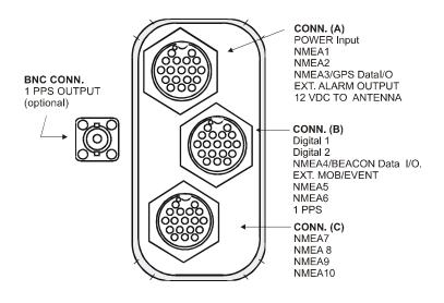
Figure 4.13 MX420/8 Rear Panel Connectors
