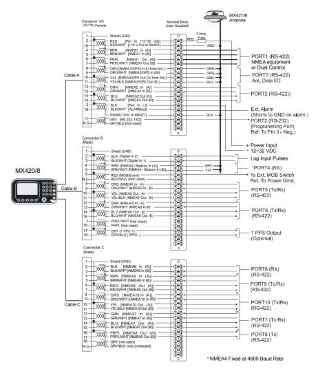
Figure 4.4 MX420/8 Wiring Diagram
