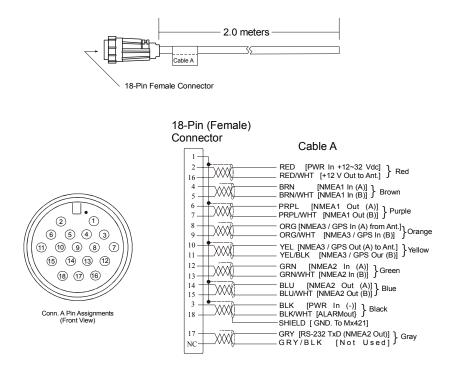
Figure 4.9 Cable (A) Wiring Configuration
