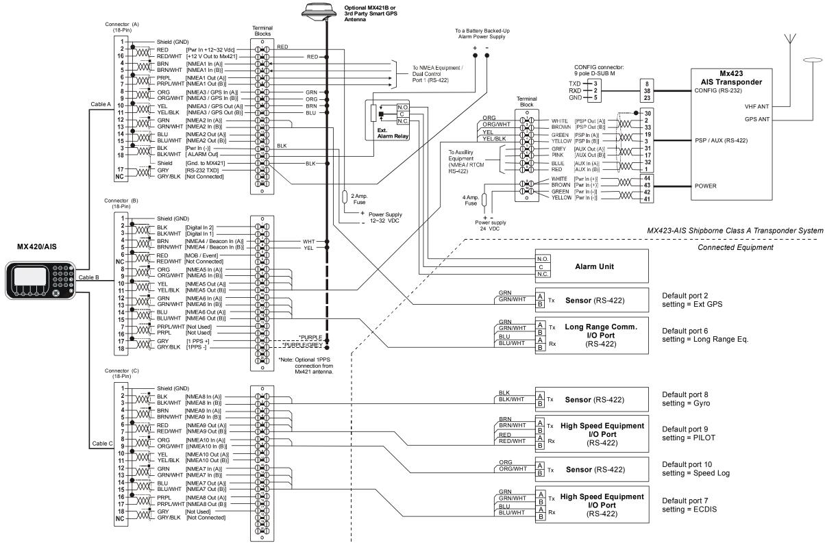
Figure 4.18 MX420/AIS CDU & MX423 (SAAB) Transponder System Wiring Diagram
