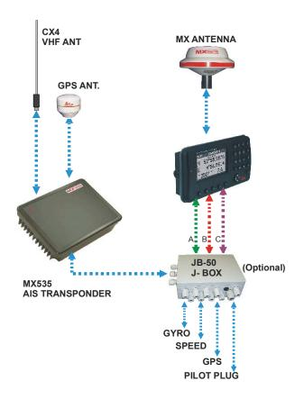
Figure 4.21 MX420/AIS/MKD CDU & MX535 (NAUTICAST) Transponder Block Diagram
