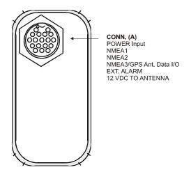
Figure 4.12 MX420/2 Rear Panel Connector
